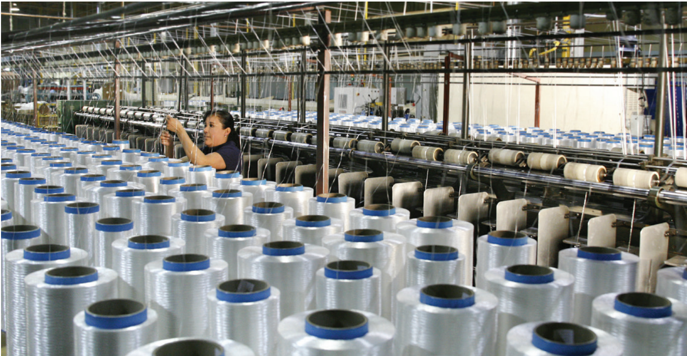
The ring twister combines multiple piles of high tenacity filament polyester yarns.
